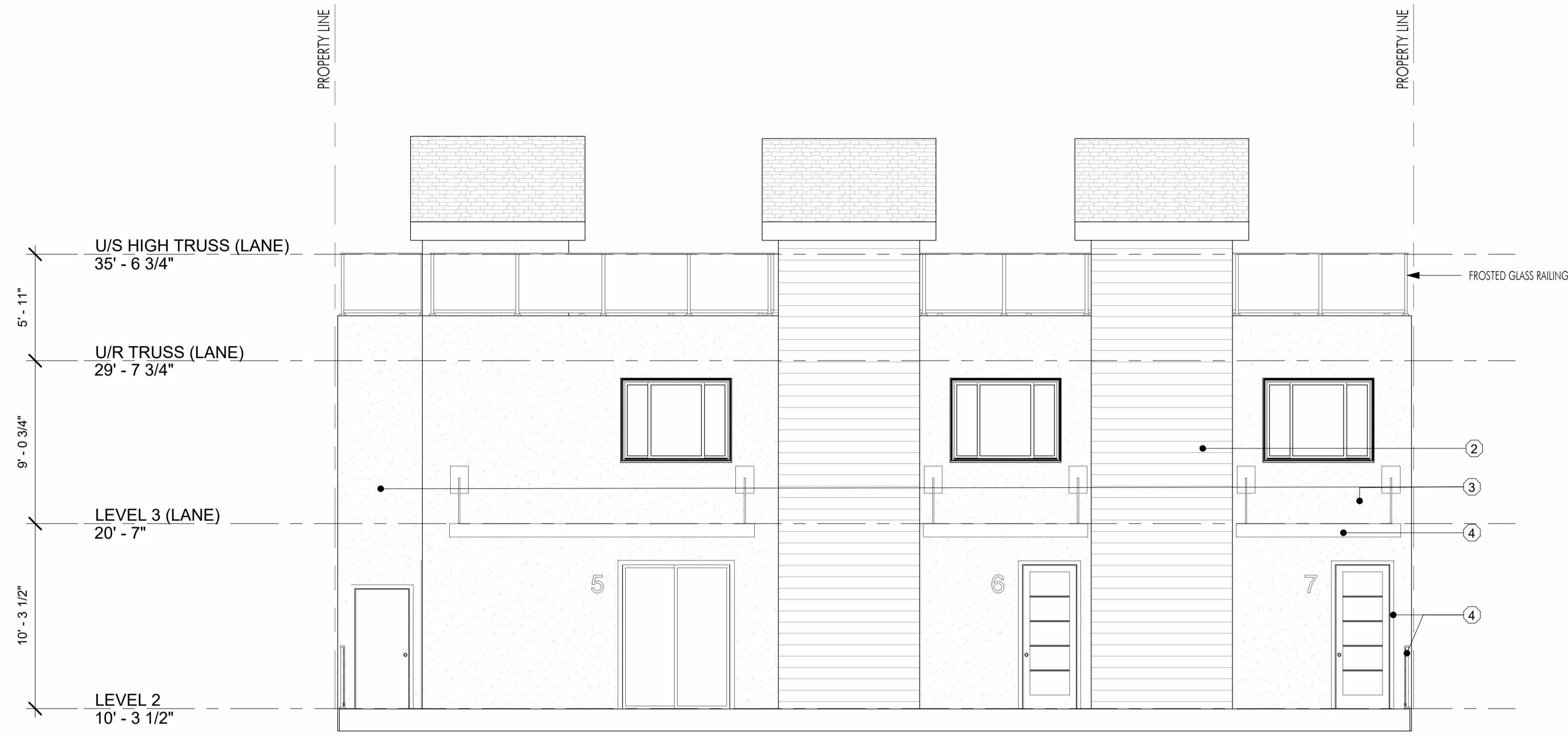
1 COURTYARD ELEVATIONS UNITS 5-7 A-205 3/16" = 1'-0"
