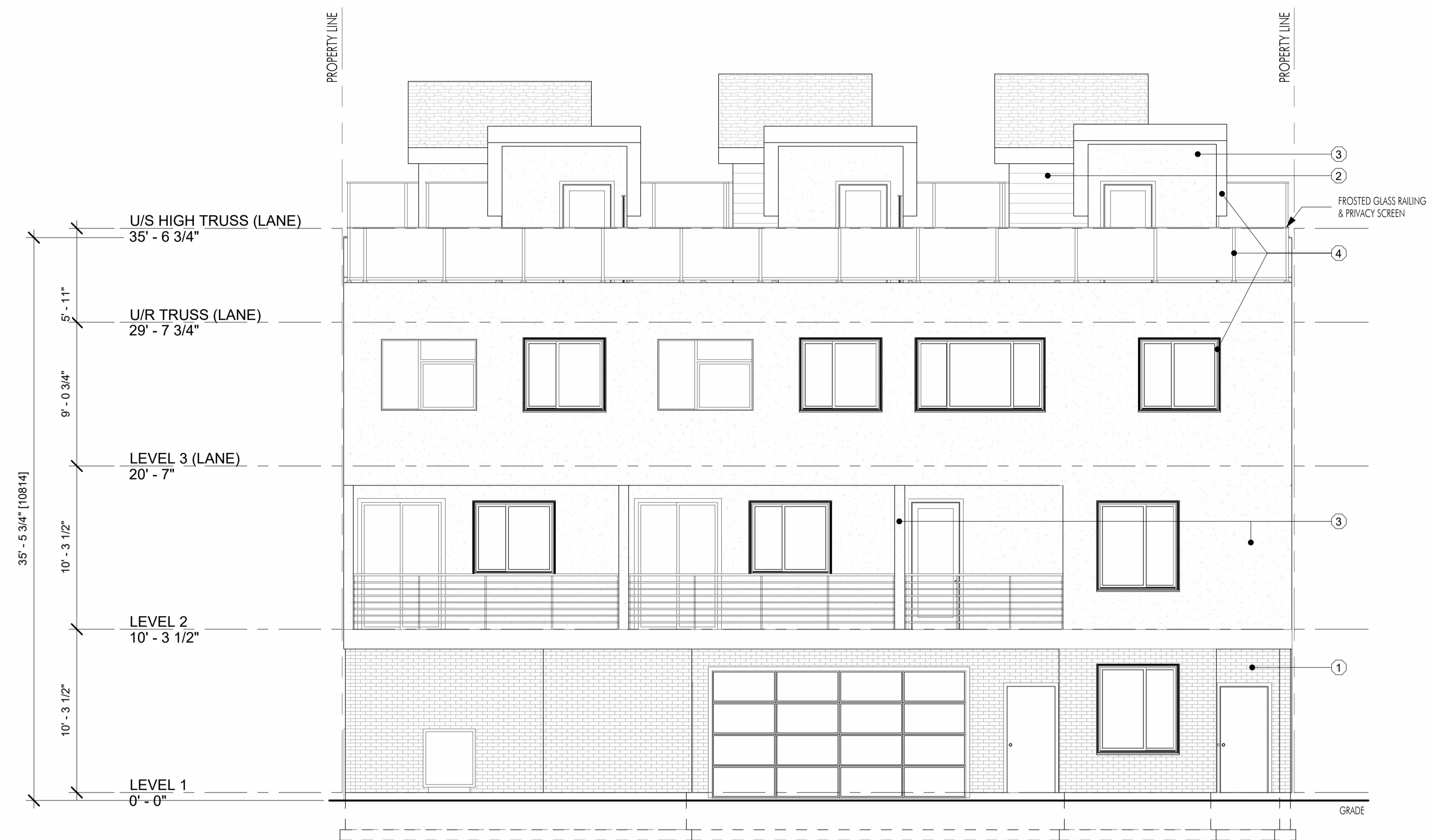
1 BACK ELEVATION A-202 3/16" = 1'-0"
