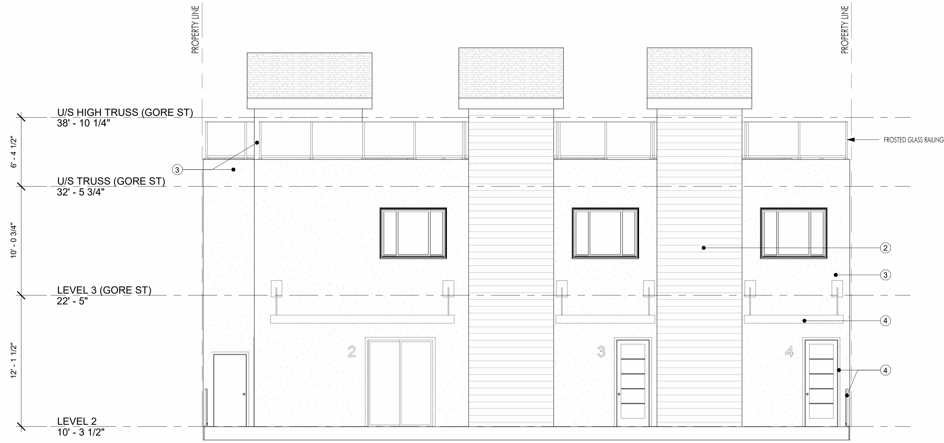
1 COURTYARD ELEVATIONS UNITS 2-4 A-204 3/16" = 1'-0"
