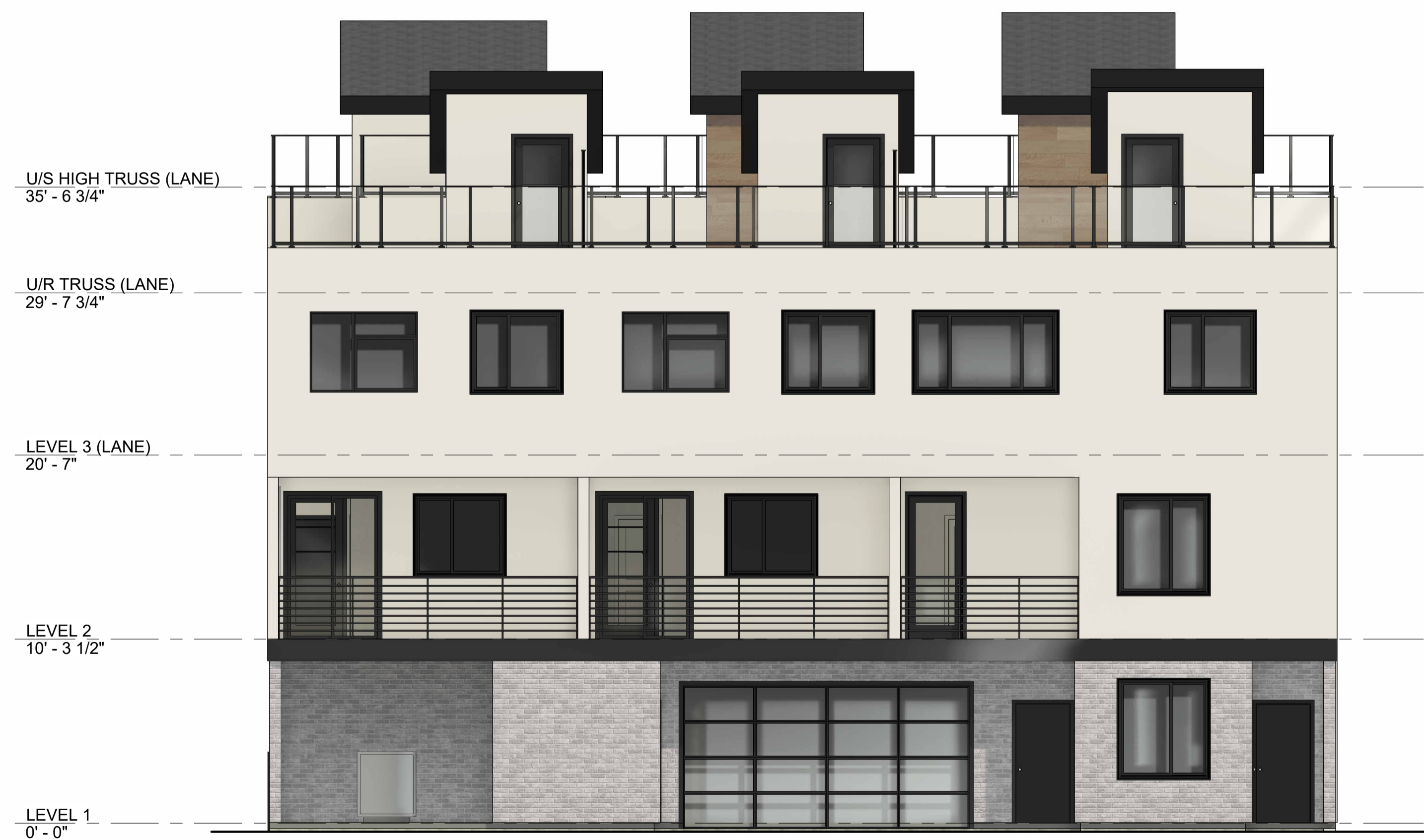
2 BACK ELEVATION (COLOUR) A-202 3/16" = 1'-0"
