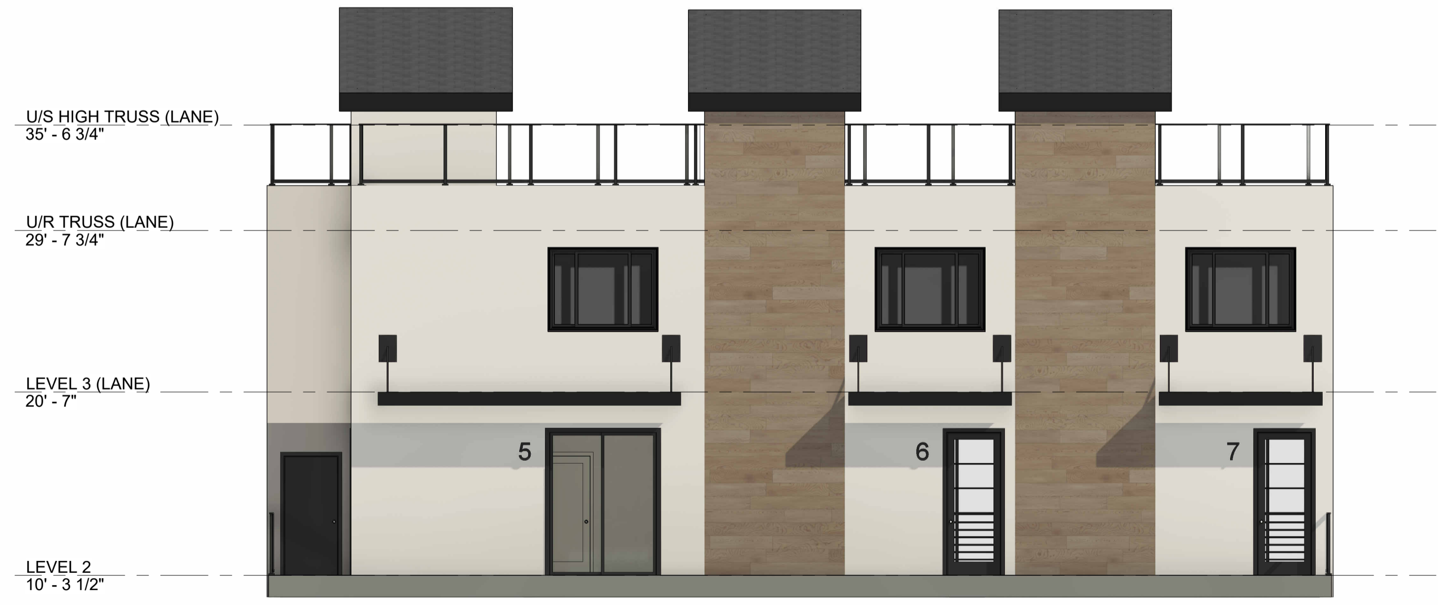
2 COURTYARD ELEVATIONS UNITS 5-7 (COLOUR) A-205 3/16" = 1'-0"
